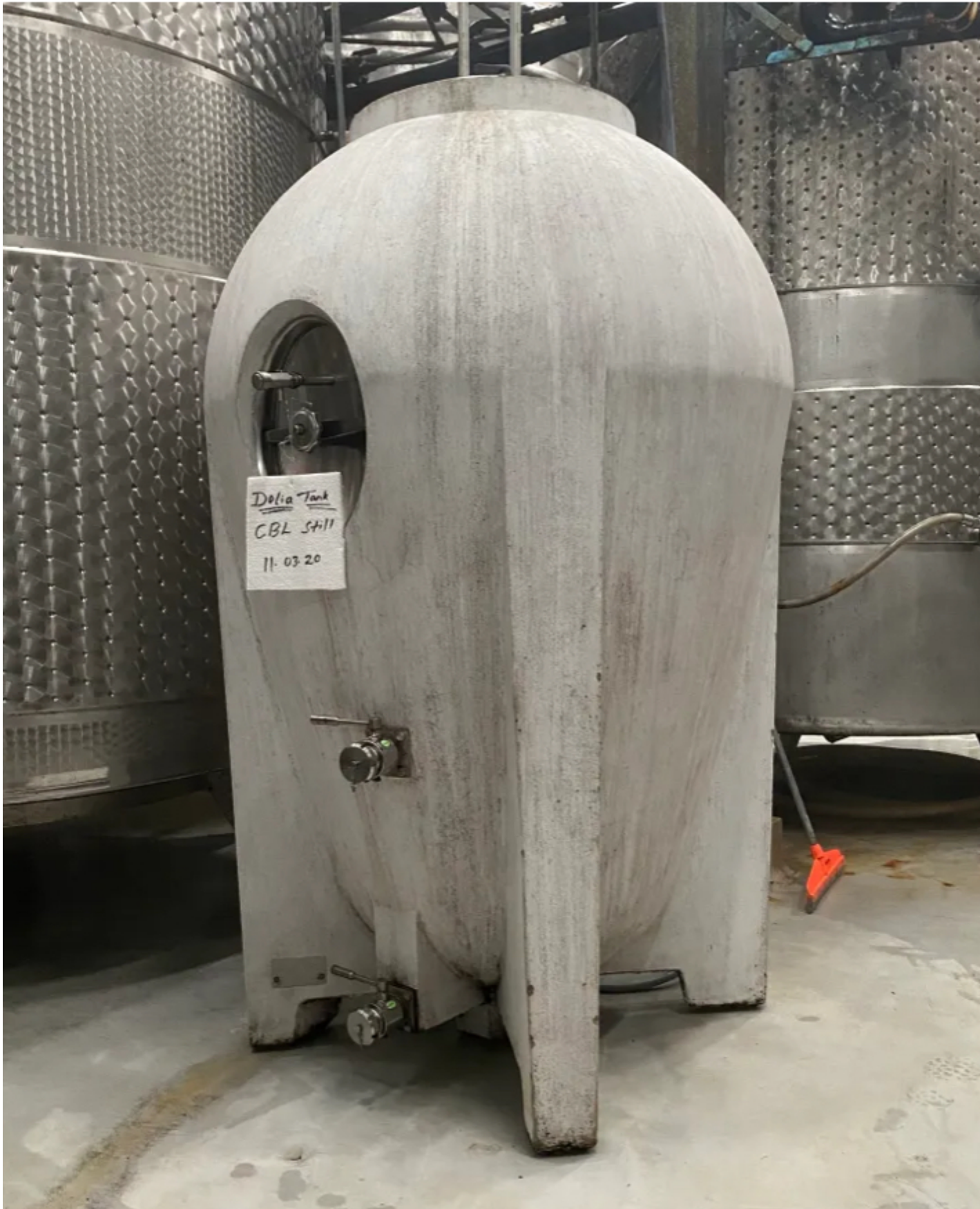
A Concrete tank at Grover Zampa Vineyards
