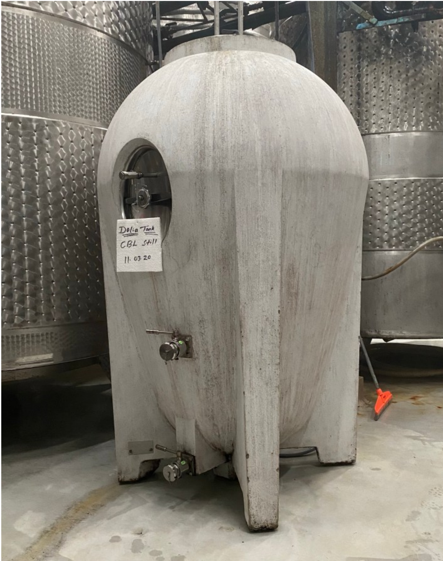
Concrete tank is becoming a preferred choice for fermentation by many wineries
